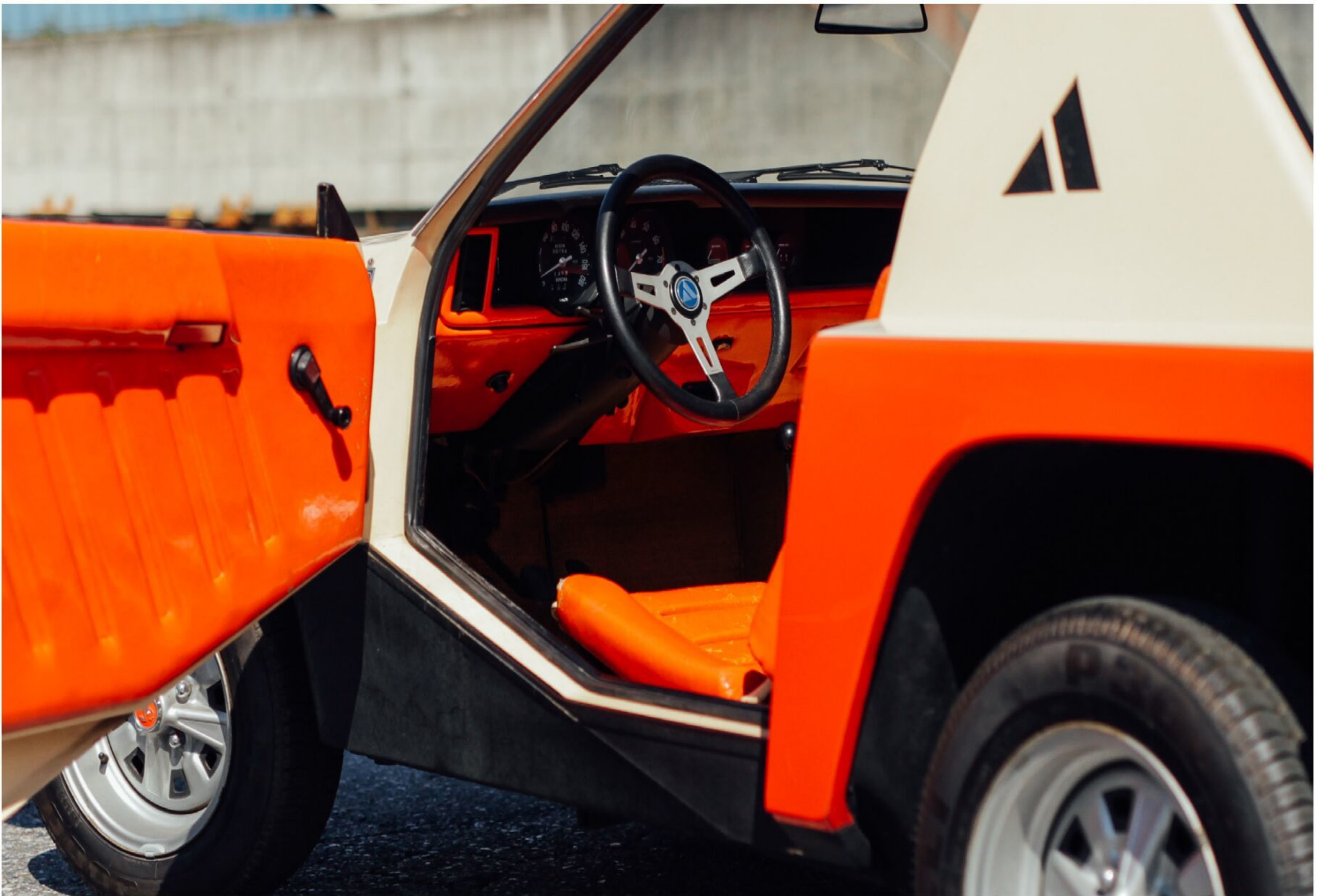
THIS PAGE: The minimalist theme continued inside the car, where the three-spoke steering wheel and five analogue gauges were sourced straight from the A112 parts bin.
